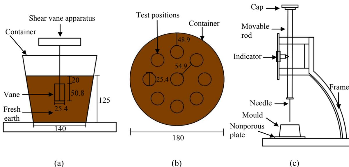
**Figure 2.** Experimental procedure diagrams: (a) Side view of shear vane tests; (b) Plan view of shear vane tests with measuring points; (c) Vicat needle tests.
