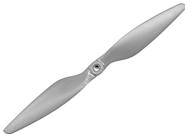
Figura 8 Hélice LP 10045MR 10X4.5 MRP, marca APC [30].
