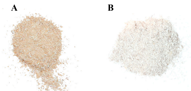
Figure 1. The physical appearance of crown pineapple fiber before (A) and after (B) chemical treatment.
