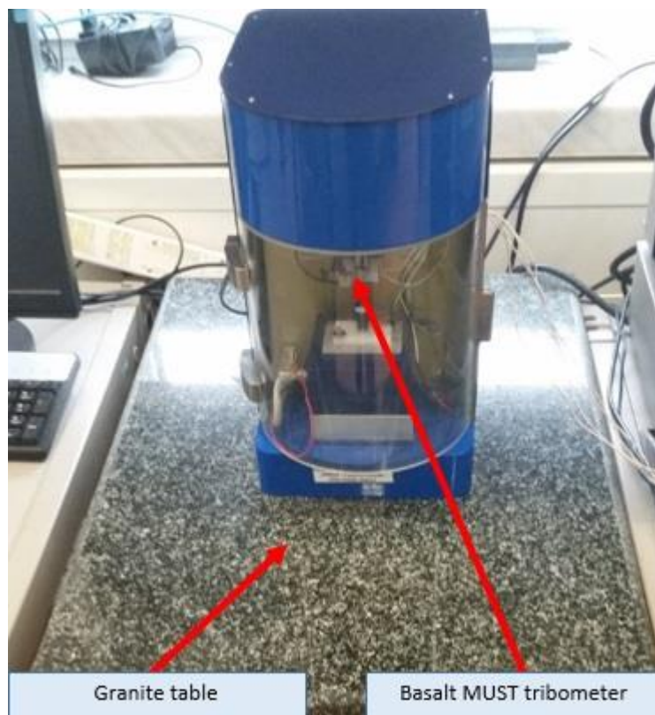
Figure 92: Work space for the Basalt MUST tribometer free from any wire, tool or object.
