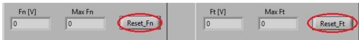
Figure 71: Finding peak values. The buttons "Reset_Fn" and "Reset_Ft" resets the "Max Fn" and "Max Ft" respectively
