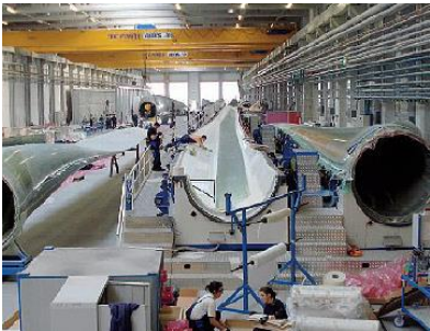
Automated wind power blade manufacturing line.
