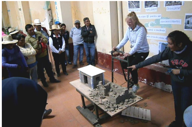
Figure 6. Dynamic test with the portable shaking table.
