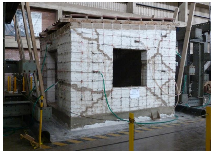
Figure 3. Full-scale adobe model reinforced with nylon rope mesh.
