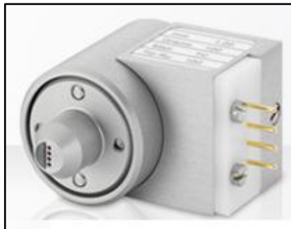
Figure 4-4. Four probes head of the NAPSON equipment.
