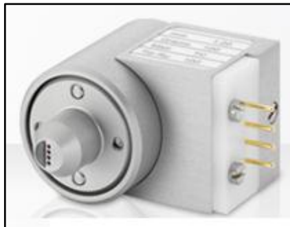
Figure 4-4. Four probes head of the NAPSON equipment.
