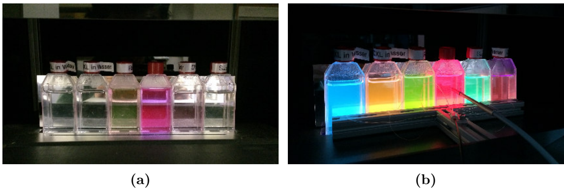
Figure 6.5: Dyomics Dye Marker (a) Liquids with natural light (b) When the fluids receive Ultraviolet light (UV), these have a emission in a certain wavelength, optical fiber of both spectrometer are located in front of bottles to inspect their behavior
